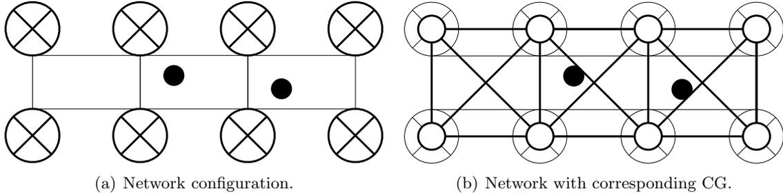
Figure 14: Fig. 14(a) shows an example sensor network with eight sensors ( $\otimes$ ) and two targets ( $\bullet$ ). Fig. 14(b) shows the corresponding CG representing the agent dependencies. The graph has an average degree of 4, and an induced width of 3.
