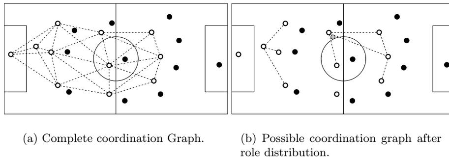
**Fig. 1.** After observing the ball position and knowing the ball position, the coordination graph is simplified considerably.
